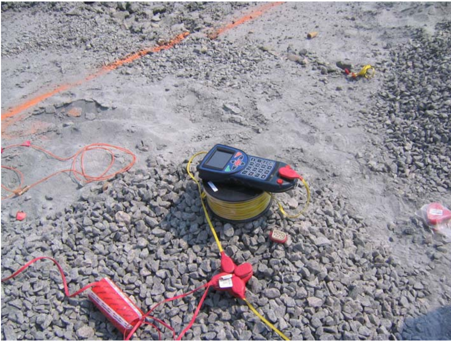
Figure 7 - Bench controller connects all rows and branches on bench
