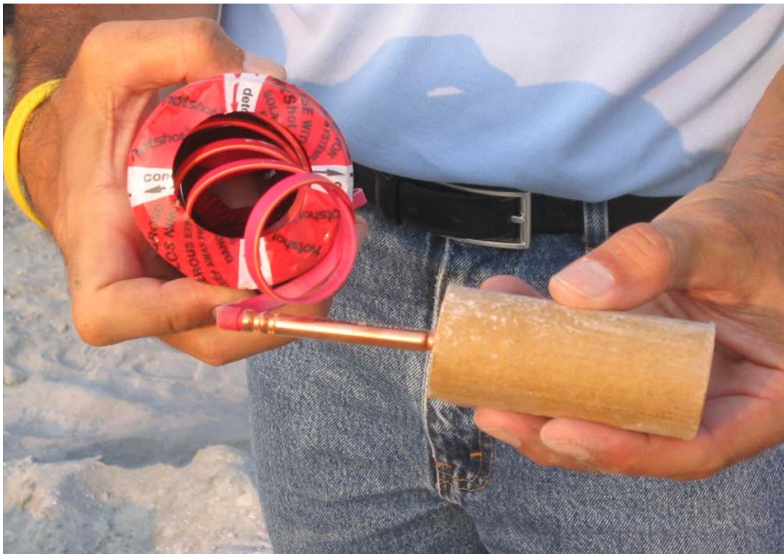
Figure 4 - HotShot electronic detonator, cardboard sheath and connecting wire
