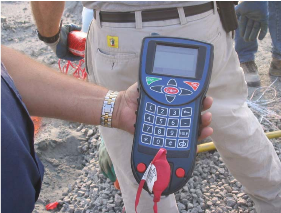
Figure 5 - HotShot Tagger showing plug connection to detonator wire
